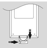
Put a CR2025 lithium battery (3V) into the compartment. Make sure the + polarity is face up.
